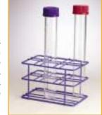
easy cleaning and is steam autoclavable at 121°C (250°F). Rack is 130mm (51/8") high, holes are 42mm square for 40mm diameter bottles.
